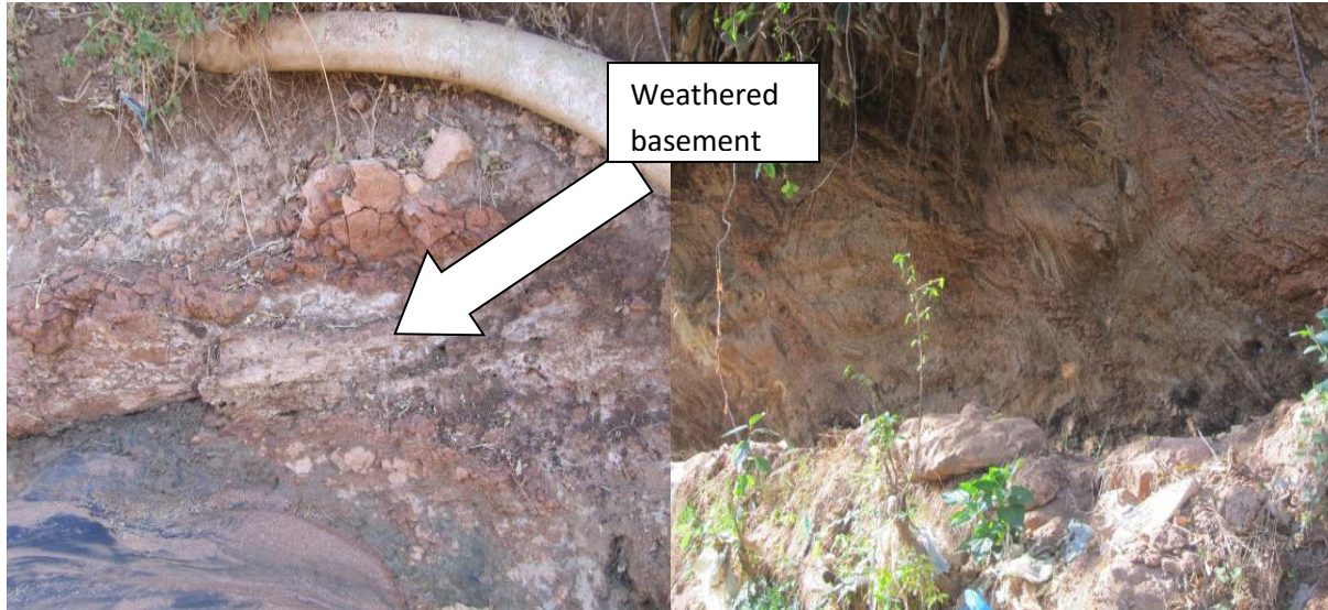
Figure 3: Fractured and weathered basement rocks along the canal route
